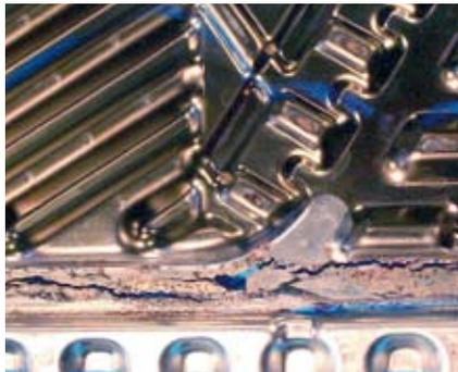
The wrong gaskets or poor gluing can cause leakage. The wrong glue may even destroy the plate.
