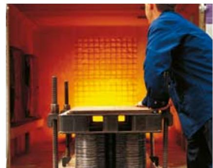
We use an oven-cured, two-component epoxy for PHEs that are frequently opened, so that gaskets stay in place after countless openings.
