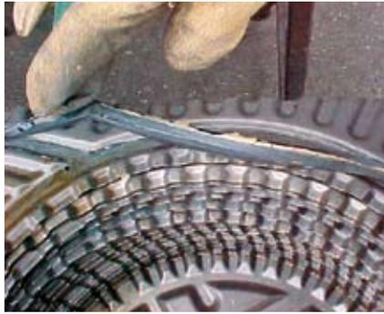
When old glue and gaskets are not completely removed, insufficient sealing is the result. This creates a high risk of leakage.
