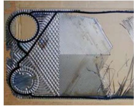
Chemical cleaning requires the right concentration, temperature and cleaning time. Otherwise, the plates can be destroyed.
