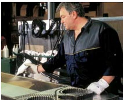
Alfa Laval gaskets and glues are specially formulated for their applications, thus ensuring an optimal alignment and seal.
