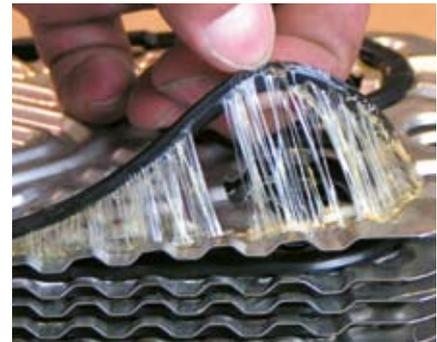
If standard glue is used on a frequently opened PHE, the gaskets may fall off, making it necessary to re-gasket after opening.
