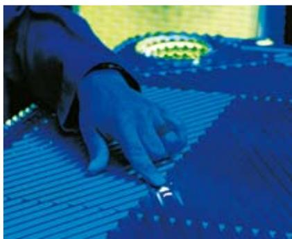
We search for pinholes and deformities with advanced techniques, including dye penetrants and UV illumination. This lets us find even the smallest crack
