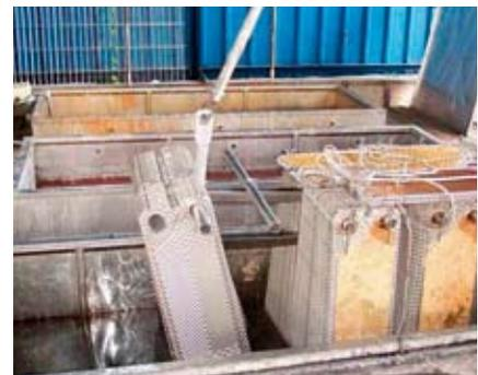
To ensure the perfect cleaning cycle, we rely on specially designed hydrojet cleaning or specialized chemical baths with the right concentration and temperature.
