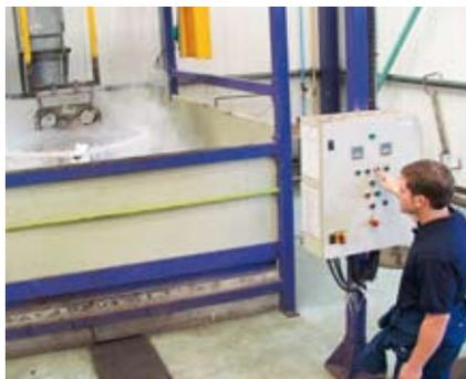
With media such as liquid nitrogen and caustic soda, we remove gaskets gently and completely, leaving the groove intact.
